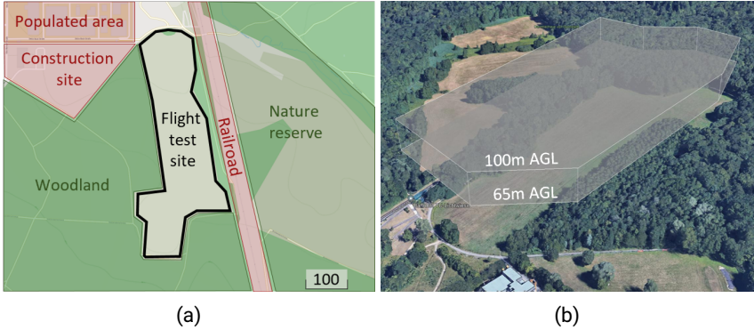
Figure A.6.: Location of the flight test site of the TU Darmstadt, based on openaip 1 (a) and implemented geofence to control the operational volume, based on [Joe22] and google earth 2 (b)
