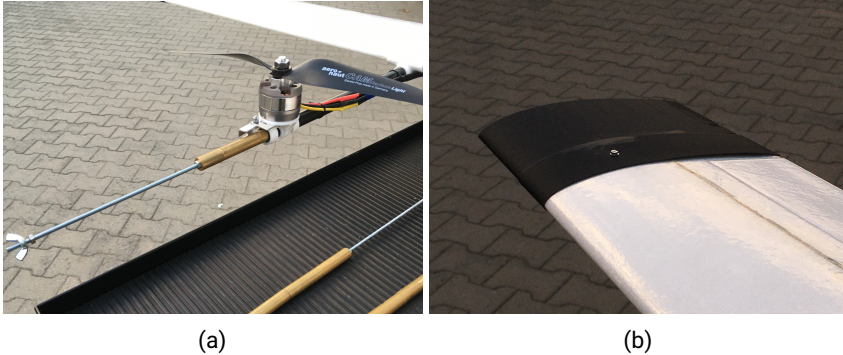
Figure A.5.: Mounting of weight modules on the right wing of the UAS (a) and the mounted lift module on the right wing tip (b) [Fic+20].
