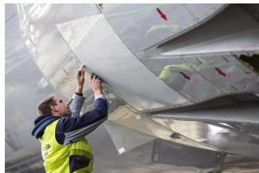
(b) Application of sharkskin on an aircraft fuselage, with permission from [Luf19]
