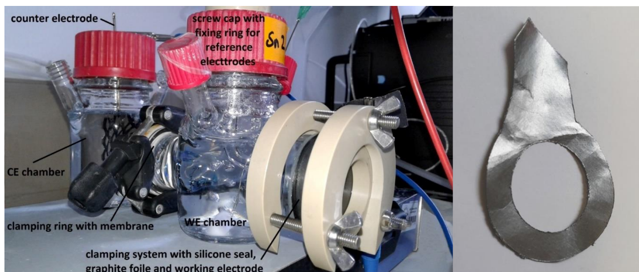
Figure S10: Mounted H-cell without reference electrode (left), ready-cut graphite foil for electrical contacting of the working electrode (right), the graphite foil is placed between the silicone seal and the working electrode.
