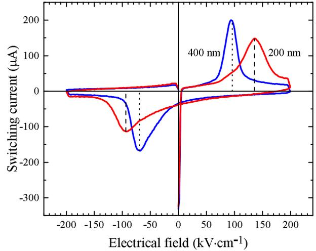
FIG. S2. Switching current versus electric field hysteresis loops at 100 Hz of 200 nm and 400 nm thick PZT layers of PZT/LNO/Al<sub>2</sub>O<sub>3</sub>/Pt/SS304 samples, respectively. The datasets used were the same as their respective  $P$ - $E$  loops plotted in Fig. 5 of the article. The dashed lines indicates the position of the positive and negative coercive fields of 200 nm and 400 nm thick PZT films, respectively.
