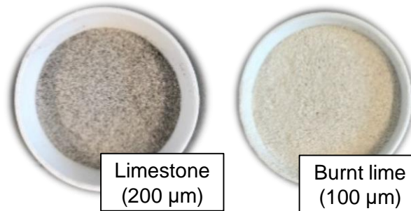
Samples from the pilot testing at 300 kW th scale. © EST Institute, TU Darmstadt.
