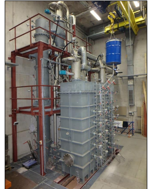
300 kW th IHCaL pilot testing facility scale. © EST Institute, TU Darmstadt.
