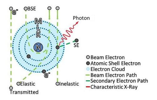
Figure 3.3: Schematic description of how an electron beam interacts with an atom (nucleus and electron cloud) in a sample. The figure shows the elastic/inelastically scattered electrons as well as the transmitted ones. Secondary electrons are electrons generated as ionization products. They produce characteristic photons. Back-scattered electrons are electrons that are scattered backward due to the strong positive charge of the nucleus. The figure is reshaped from Ref. <sup>[166]</sup>.
