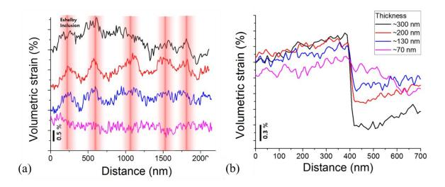
Figure 4.9: Line profiles of the volumetric strain maps (a) along the SB1 and (b) perpendicular to SB2 in the directions indicated by dash arrows in Figure 4.8c-f for different thicknesses of about 300 nm, 200 nm, 130 nm, and 70 nm.
