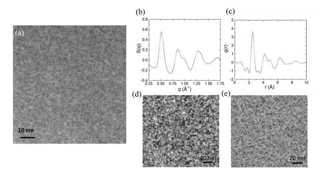
Figure 4.3: STEM-PDF analysis for characterization of as-spun  $Fe_{85.2}Si_{0.5}B_{9.5}P_4Cu_{0.8}$  metallic glass ribbons. (a) a STEM-HAADF image. (b) Averaged structure factors and (c) averaged PDFs from the STEM-PDF data cube. (d) Maps for the first peak intensity of S(q)s and PDFs.
