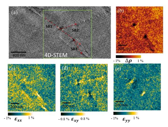
Figure 7.7: Secondary shear bands and their brunching points in the as-cast  $Zr_{46}Cu_{38}Al_8Ag_8$  bulk metallic glass. (a) STEM-HAADF image showing the area for 4D-STEM mapping (green rectangle). (b) is a relative atomic density map. The coordinate system is defined as x-axis parallel and y-axis perpendicular to SB1 (c)-(e) are strain tensor  $\varepsilon_{xx}$ ,  $\varepsilon_{xy}$ , and  $\varepsilon_{yy}$ .
