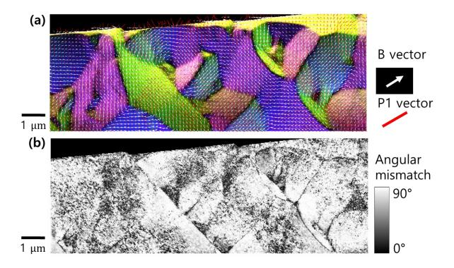
Figure 8.5:As-spun Fe<sub>85.2</sub>Si<sub>0.5</sub>B<sub>9.5</sub>P<sub>4</sub>Cu<sub>0.8</sub> metallic glass ribbon after plastic deformation. (a) Vector field visualization of the magnetic moments  $(B_x, B_y)$  with white arrows and the first principal strain  $(\varepsilon_{1x}, \varepsilon_{1y})$  with red sticks overlayed by the color map of  $\vec{B}$ . (b) Angular mismatching between  $\vec{B}$  and  $\vec{\varepsilon}_1$ .
