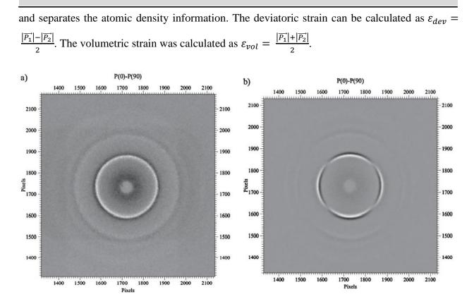
Figure 3.10: Difference between the 2-D XRD pattern measured in two orientations  $P(0^{\circ})-P(90^{\circ})$  for a Fe-based metallic-glass sample annealed at 300°C (a) without stress (b) under stress. The sample annealed under stress undergoes creep and is expected to be similar to shear-band material; it shows anisotropy after unloading indicating the presence of residual stress within the material after deformation. Reprinted from Ref. <sup>[176]</sup>.
