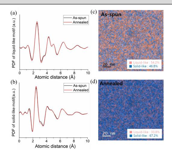
Figure 5.4: Atomic structure mapping of the as-spun and annealed Fe<sub>85.2</sub>Si<sub>0.5</sub>B<sub>9.5</sub>P<sub>4</sub>Cu<sub>0.8</sub> metallic glasses using NMF-aided STEM-PDF analysis. Basis PDFs of (a) the liquid-like and (b) the solid-like structural bases separately obtained from both as-spun and annealed metallic glass samples. Maps of the liquid-like and solid-like structural bases for (c) as-spun and (d) annealed samples with the fraction of each structural type indicated.
