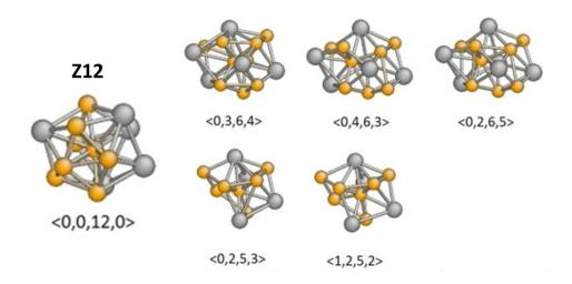
Figure 2.3: Distorted Z12 clusters due to topological restrictions. Voronoi tessellation allows for cluster distortion with deviations in atomic bond lengths by altering the coordination number. Examples include the Z12 cluster being distorted to <0,3,6,4>, <0,4,6,3>, <0,2,6,5>, <0,2,5,3>, as <0,1,5,2>. Reprinted from Ref. <sup>[21]</sup>.
