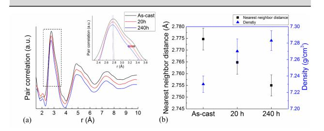
Figure 7.1: (a) Electron PDF calculated from SAED pattern of the as-cast, 20 h, and 240 h annealed  $Zr_{46}Cu_{38}Al_8Ag_8$  metallic glasses. The first peaks of PDFs are enlarged in the inset. The heights of the PDFs are normalized by their first peak and displaced for easy presentation of peak shifts. The first peak positions of the first peak in the PDFs correspond to the nearest atomic neighbor distance, which is plotted in (b) together with mass density measured by Archimedes' principle.
