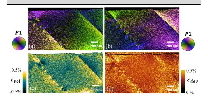
Figure 4.6: Deformed Fe<sub>85.2</sub>Si<sub>0.5</sub>B<sub>9.5</sub>P<sub>4</sub>Cu<sub>0.8</sub> metallic glass ribbon. (a) first principal strain,  $P_1$ , (b) second principal strain,  $P_2$ , (c) volumetric strain, and (d) deviatoric strain.
