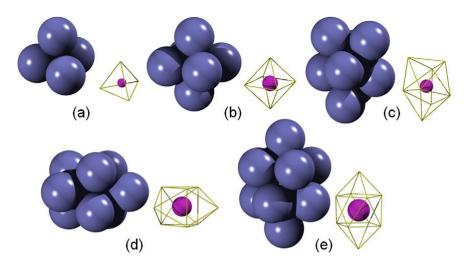
Figure 2.1: The DRPHS model proposes five fundamental structures: (a) tetrahedron, (b) octahedron, (c) tetragonal dodecahedron, (d) trigonal prism capped with three half octahedra, and (e) Archimedean antiprism capped with two half octahedra. Reproduced from Ref. <sup>[25]</sup>.
