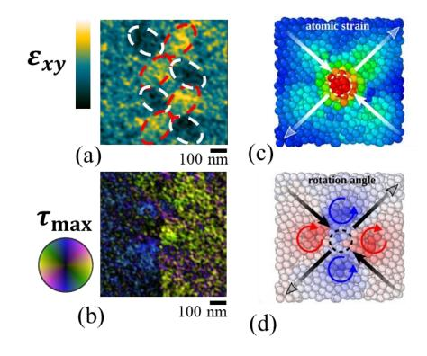
Figure 6.3: Visualization of an Eshelby quadrupolar strain field. Experimental data of (a) shear strain  $\varepsilon_{xy}$  and (b) maximum shear strain  $\tau_{max}$  in a Fe<sub>85.2</sub>Si<sub>0.5</sub>B<sub>9.5</sub>P<sub>4</sub>Cu<sub>0.8</sub> metallic glass ribbon obtained from 4D-STEM strain mapping and MD simulation of a STZ from Ref. <sup>[207]</sup> for (c) atomic strain and (d) rotation angle.
