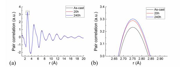
Figure 7.2: (a) Synchrotron Synchrotron-based X-ray pair distribution function analysis of the ascast, 20 h, and 240 h annealed  $Zr_{46}Cu_{38}Al_8Ag_8$  metallic glasses obtained from synchrotron radiation X-ray diffraction. The first peaks of each PDF are enlarged in (b).
