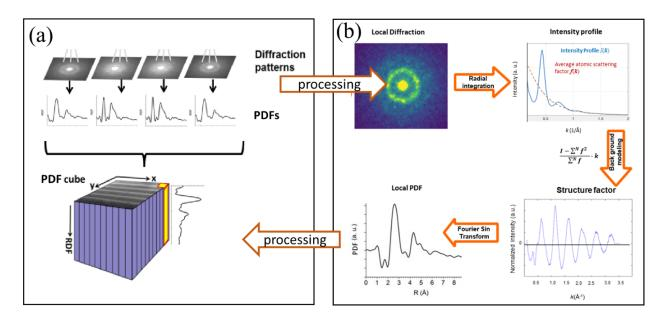
Figure 4.2: Schematic illustration of STEM-PDF mapping. (a) Local diffraction patterns and corresponding PDFs acquired by microprobe 4D-STEM setup. (b) The diffraction patterns are individually processed into a PDF cube. Reprinted from Ref.<sup>[172]</sup>.
