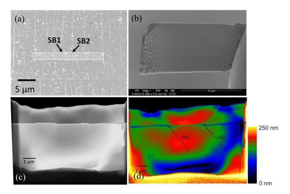
Figure 3.7: Cross-sectional TEM sample preparation by dual-beam SEM-FIB system. (a) milling trenches from the area of interest, (b) TEM lamella after lift-out before thinning, (c) after thinning for electron transparency, STEM-HAADF image, and (d) Thickness map of a typical TEM lamella for investigation obtained from energy-filtered transmission electron microscopy (EFTEM).
