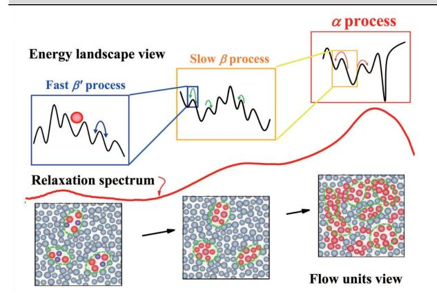
Figure 2.5: Schematic representation of relaxation processes in metallic glasses, depicting the potential energy landscape and atomic configurations. The many-body potential energy is illustrated as a function of atomic distances. Active atoms are represented by red color, and atoms surrounded by green dashed circles represent flow units. Modified from Ref.<sup>[84]</sup>.
