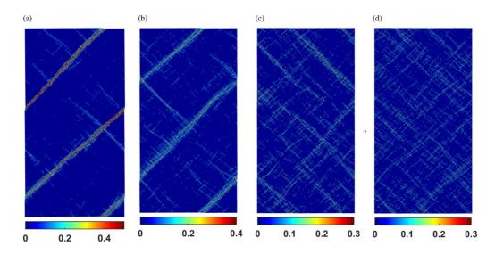
Figure 2.11: Influence of nanoscale structural heterogeneity on shear banding in metallic glasses. Shear band generation in a metallic glass with different amounts of the STZ volume fractions (a) 0%, (b) 10%, (c) 20%, and (d) 30%. Reprinted from Ref. <sup>[127]</sup>.
