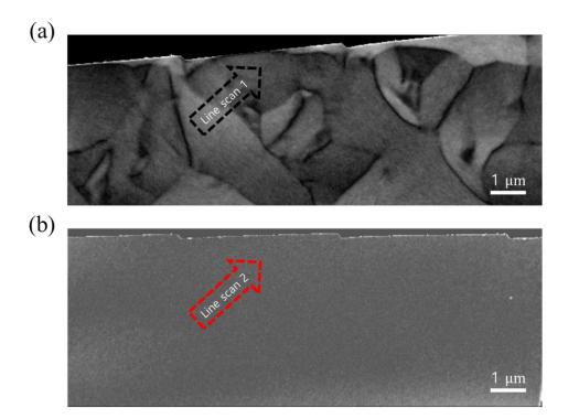
Figure 8.4: Map of the strength of DPC signal from (a) unmagnetized (Ltz-condition), and fully magnetized (conventional STEM condition)  $Fe_{85.2}Si_{0.5}B_{9.5}P_4Cu_{0.8}$  metallic glass ribbon. (c) Line profiles taken across the shear band from the measurements of (a) Ltz-condition indicated by a black dash arrow (Line scan 1) and (b) conventional STEM condition indicated by a red dash arrow (Line scan 2).
