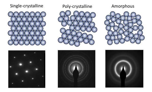
Figure 3.8: Schematic illustration of typical atomic structures of solids, *e.g.* single crystal, polycrystal, amorphous, and corresponding electron diffraction patterns.
