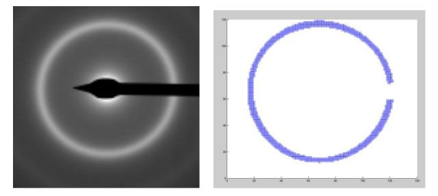
Figure 4.5: A typical diffraction pattern of Fe<sub>85.2</sub>Si<sub>0.5</sub>B<sub>9.5</sub>P<sub>4</sub>Cu<sub>0.8</sub> metallic glass (left) which was binarized using a threshold with  $I(q_x,q_y) = 1$  for  $0.95I_{max} < I(q_x,q_y) < I_{max}$  and 0 everywhere else (right).
