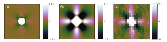
Figure 2.7: STZ structure with the strain field around it (a) Calculated shear strain field at STZ subjected to a strain of 0.05. (b) Autocorrelation function of (a). (c) Experimentally measured self-correlation of the strains in a colloidal glass. Reprinted from Ref. <sup>[98]</sup>.
