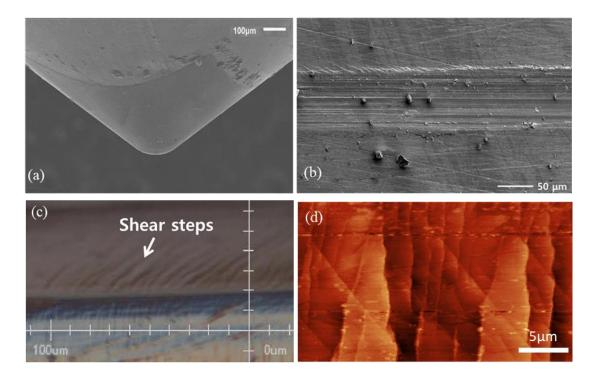
Figure 3.2: SEM images of (a) tip and (b) scratched track with wear debris and shear offsets on the pile-up area. The scratches were imaged by (c) optical microscopy and (d) atomic force microscopy.
