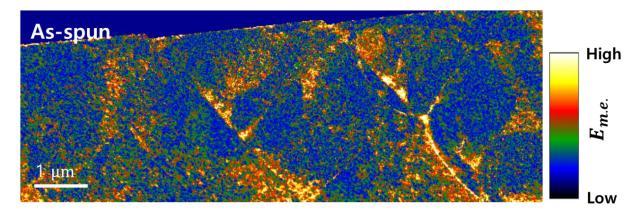
Figure 8.7: Map of magnetoelastic energy of the as-spun  $Fe_{85.2}Si_{0.5}B_{9.5}P_4Cu_{0.8}$  metallic glass ribbons after deformation.
