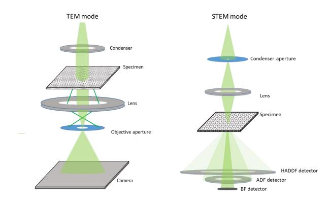
Figure 3.6: Schematic view of conventional TEM and STEM modes.
