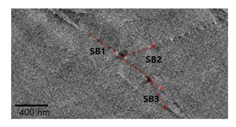
Figure 6.6: STEM-HAADF images showing secondary shear bands and their brunching points in  $Zr_{46}Cu_{38}Al_8Ag_8$  bulk metallic glass. SB2 exhibits alternating fluctuation with a much shorter distance (< 100 nm).
