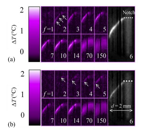
Figure 2.12: Heat generation during shear banding observed by infrared (IR) thermography. (a) The instantaneous appearance of the shear band, and (b) propagating heat front; Numbers indicate the frame number, whereby one frame is measured within 0.4 ms. Reprinted from Ref. <sup>[139]</sup>.
