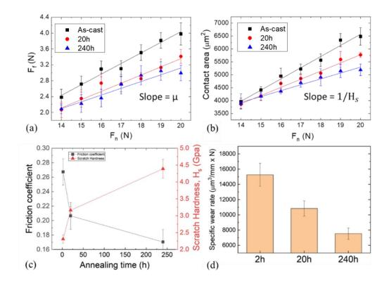
Figure 7.4: Tribological response of as-cast, 20 h, and 240 h annealed  $Zr_{46}Cu_{38}Al_8Ag_8$  bulk metallic glasses. Load dependence of (a) friction force used to determine the friction coefficient as the slope and (b) of contact area used to determine the scratch hardness from the reciprocal slope; (c) friction coefficient and scratch hardness as a function of annealing time and (d) bar graph of specific wear rate.
