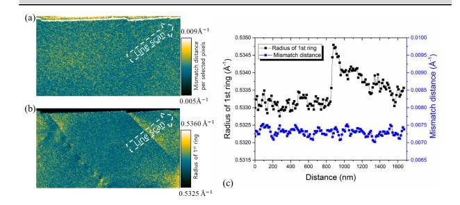
Figure 4.7: Statistical analysis for the accuracy of the strain measurement. (a) Map of fitting error for strain measurement. (b) Map of the radius of the 1<sup>st</sup> ring ( $q_{max}$ ). (c) Line profiles of the mismatch distance and the radius of the 1<sup>st</sup> ring in the region indicated by white dash arrows in (a) and (b).
