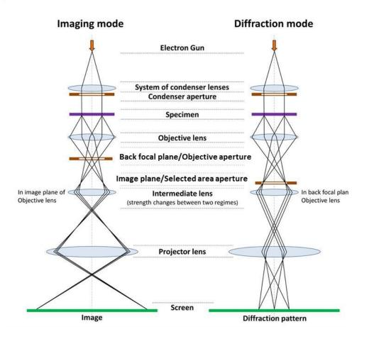
Figure 3.5: Schematic view of the imaging and diffraction mode of TEM. Reprinted from Ref.<sup>[166]</sup>.
