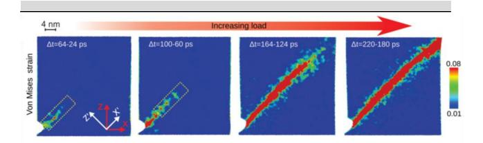
Figure 2.10: Time-dependent progression of a shear band. Structural variations are depicted by Von Mises strain in the simulated metallic glass during the early stages of shear banding. The figures are reprinted from Ref.<sup>[120]</sup>.
