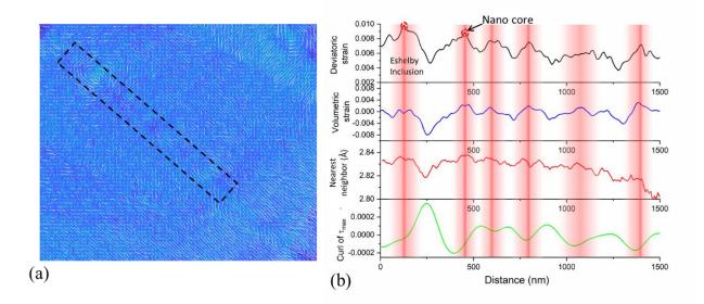
Figure 6.5: (a) Vector field visualization of the maximum shear strain overlayed on the atomic density map for a  $Zr_{46}Cu_{38}Al_8Ag_8$  bulk metallic glass. (b) Line profile of relative atomic density ( $\Delta\rho$ ), deviatoric strain, volumetric strain, and curl of  $\tau_{max}$  taken along the shear band in the region indicated by a black dashed rectangle in (a). The red highlights indicate the position of the shear transformation inclusions.
