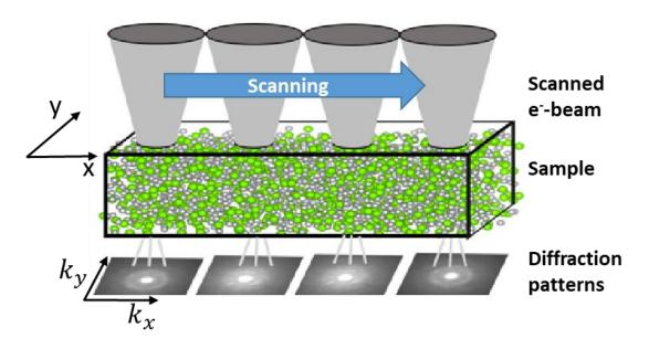
Figure 4.1: Schematic illustration of 4D-STEM. A quasi-parallel electron probe is focused to the nm scale on an electron transparent sample. Electron diffraction patterns are acquired from the nano-volume at each scan position during stepwise scanning of the probe across the area of interest. The diffraction pattern of metallic glasses is characterized by a set of circular diffraction rings due to their isotropic atomic arrangement. Reprinted from Ref. <sup>[176]</sup>.
