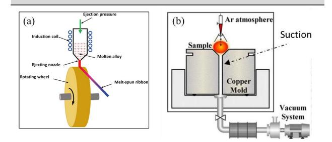
Figure 3.1: Schematic illustration of (a) a single-roller melt-spinning and (b) suction casting. Reprinted from Ref. <sup>[161]</sup> and Ref. <sup>[163]</sup>.
