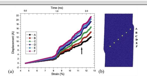
Figure 2.9: The synchronized sliding for the nucleation of shear bands in metallic glasses. (a) Displacement as a function of strain, showing the jumps in displacement (b) at the six points along the band. The figures are reprinted from Ref.<sup>[21]</sup>.
