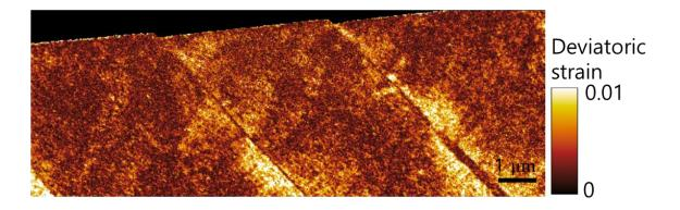
Figure 8.6: Deviatoric strain of as-spun  $Fe_{85.2}Si_{0.5}B_{9.5}P_4Cu_{0.8}$  metallic glass ribbon after plastic deformation.
