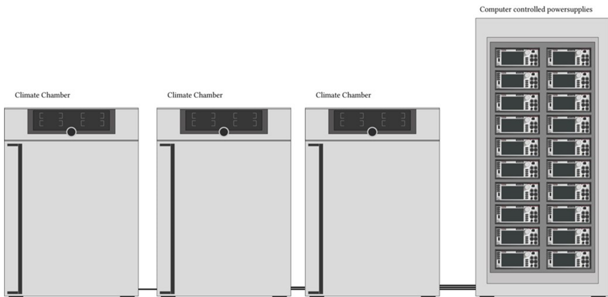
Figure 4.3: Electro-optical measurement setup for spectral and electrical LED characterization.
