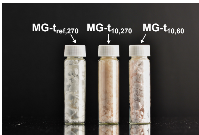
Figure 3.3: Freeze-dried reference PNIPAM microgel \text{MG-t}_{\text{ref},270} compared to P(NIPAM-co-DMA) microgels \text{MG-t}_{10,270} and \text{MG-t}_{10,60} . These P(NIPAM-co-DMA) microgels were synthesised with different total reaction times t_{\text{reac}} ( t_{\text{reac}} = 270 \text{ min} and t_{\text{reac}} = 60 \text{ min} ), but identical DMA injection times t_{\text{DMA}} = 10 \text{ min} . The reference PNIPAM microgel \text{MG-t}_{\text{ref},270} exhibits a purely white colour, while the P(NIPAM-co-DMA) microgels possess an orange to pinkish colour.
