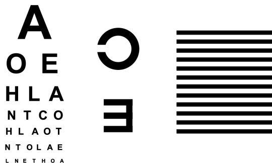
Figure 3.1.: Illustration of different test patterns for visual acuity testing listed from left to right, such as a letter chart, a Landolt ring and a Snellen E or a line pattern [76, 30].
