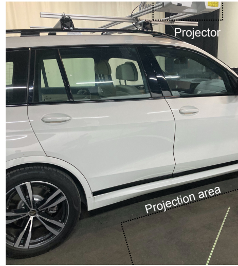
(b) Picture of the used setup, which includes a vehicle with an LCD laser projector [127] mounted via a roof construction with a projection of a line pair rotated 45^\circ . The displayed testing environment shows an ambient illuminance of 196 lux to 235 lux depending on the viewing distance to the projection.
