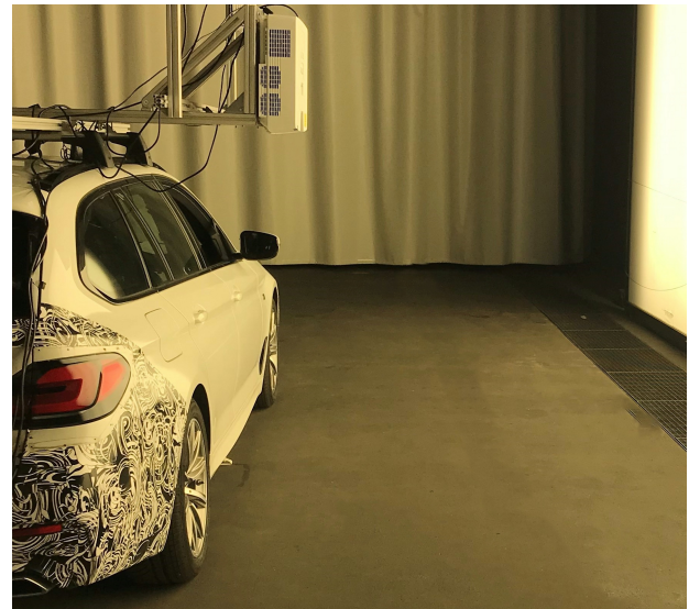
(b) Picture of the experimental setup in the DLS ( L_{\text{Background}} \approx 235 \text{ cd m}^{-2} ) with the ambient light source for the daylight-like ambient illuminance indicated on the right border of the picture.
