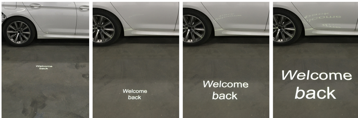
Figure 3.11.: Display of the text-based testing pattern for the SP and FR tests. From left to right: the smallest size of the plain text-based illustration from 3 m viewing distance and further the different sizes from small (27.5 cm wide x 13 cm high), middle (55 cm wide x 25.5 cm high), and big (91.5 cm wide x 42 cm high) patterns from 1 m distance. The images are taken from the perspective of the viewer.
