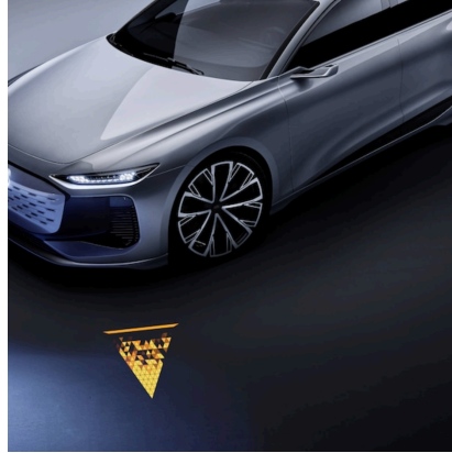
(b) Illustration of a safety-relevant projection with the example of a projected turning indicator, which shall warn or make another RU aware of a turning vehicle by projecting the amber arrow into the RU’s field of view [72].
