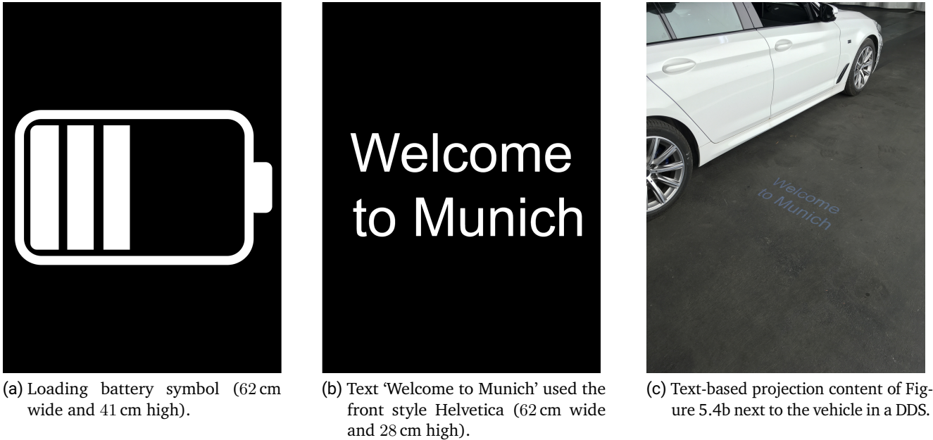
Figure 5.4.: Symbol- and text-based projection content for the perception testing, including a photo of the setup including a text-based projection.
