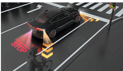
(a) Graphical illustration displays near-field projections of the vehicle's side and back [20].
