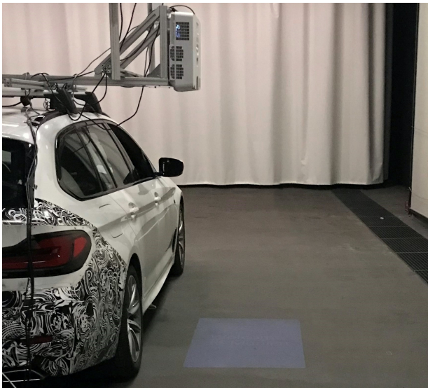
(a) Picture of the experimental setup in the PGS ( L_{\text{Background}} \approx 0.56 \text{ cd m}^{-2} ). The picture displays the car with the roof-mounted projector, which displays the projection area of the near-field projection (horizontal ( a_{\text{hor}} = 1.20 \text{ m} ) and vertical length ( a_{\text{vert}} = 0.67 \text{ m} ) of the projection).
