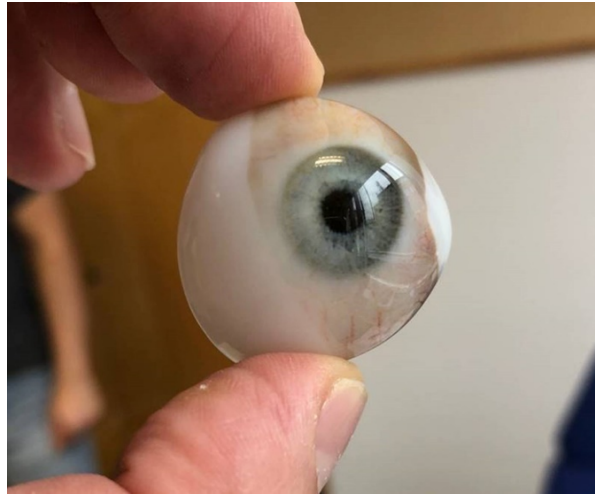
Figure B.7.: 3D printed partly-textured eye prosthesis that was polished in a post-process.
