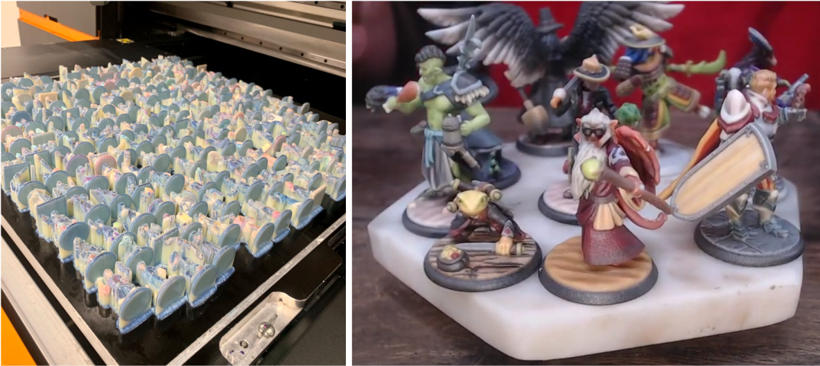
Figure 1.3.: Several 100,000 color figurine prints via Cuttlefish (A 3D printer driver developed by Fraunhofer IGD) on Mimaki 3DUJ-553 fabricated. Image rights: Hero Forge [ Herb ] (the left image) and DeadAussieGamer [ Hera ] (the right image).
