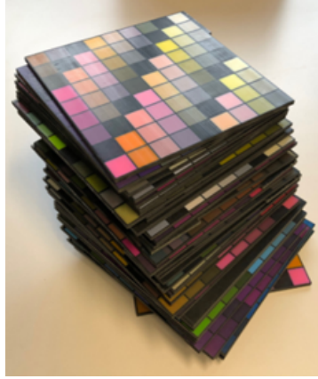
Figure B.3.: Printed target used to fit the five grid point cellular Neugebauer model to predict both color and the translucency parameter \alpha [UTB*19]
