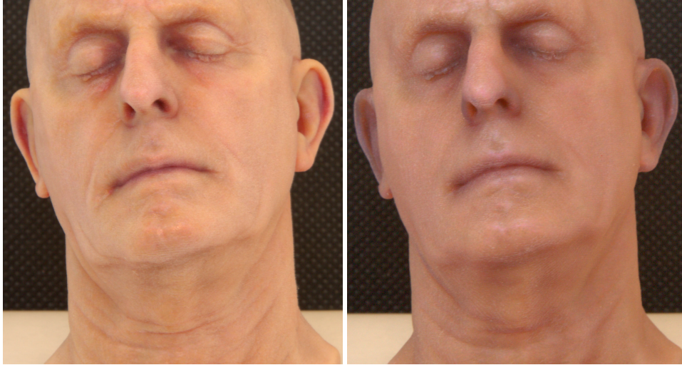
Figure B.5.: 10cm head model printed with \alpha = 0.786 (left) and \alpha = 0.518 (right). Identical model geometry and illumination conditions. Figure reproduced from Brunton et al. [BATU18].
