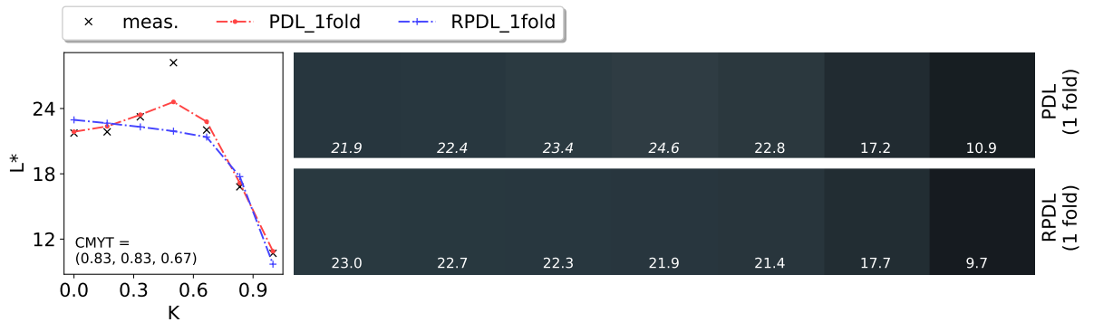
Figure 4.1.: Lightness L^* as a function of black material K with other materials fixed on a tonal case of the Mimaki 2 dataset (the fixed tonal values are shown at the lower left of the figure), and the resulting colors. The L^* values are shown as white numerical text, with italic font indicating L^* -vs- K monotonicity violations. The PDL/RPDL prediction in this figure is from a single PDL/RPDL model respectively. The figure shows that the training data itself has errors leading to monotonicity violations, and that the PDL model overfits to the erroneous data without considering monotonicity. In contrast, the proposed RPDL model ensures monotonicity despite the data outlier, indicating better robustness against errors in training data.
