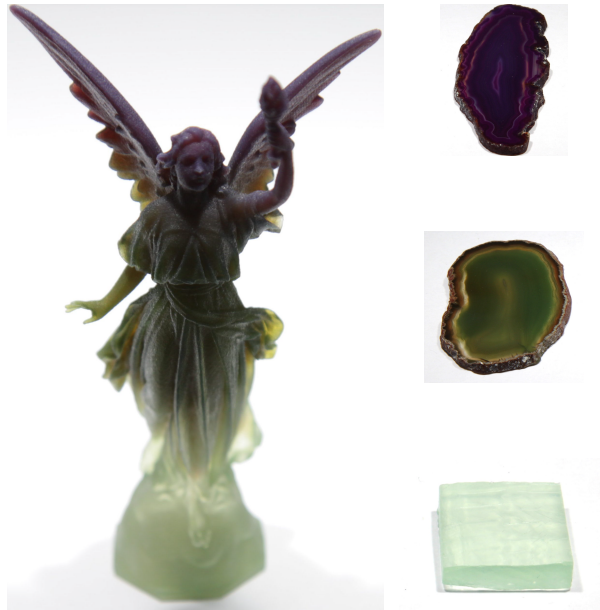
Figure B.4.: The St. Lucy model printed (10cm) with varying RGBA values. At the top is that of the violet stone, middle is green stone and bottom is green soap, with linear transitions in between. Figure reproduced from Brunton et al. [BATU18].
