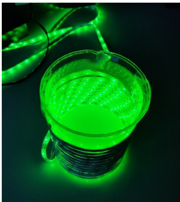
Figure 104 Home-built photoreactor for photocatalytic experiments.
