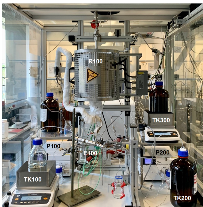
Figure 8: Front view of the laboratory fixed-bed reactor setup.
