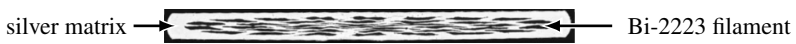
Figure 1.9.: Exemplary cross section of a multifilamentary 1 st generation HTS BSCCO wire [15]. The silver matrix is a main cost factor and restricts the cost reduction potential of 1 st generation HTS conductors.
