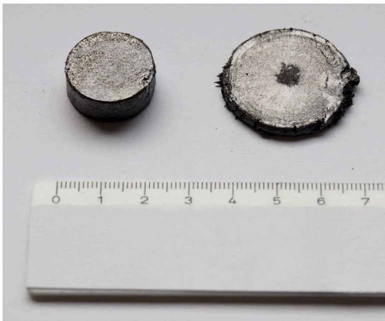
Figure S5: Appearance of the Nd-Fe-B compacts before and after Flash SPS. Due to conducting the Flash SPS cycles without an outer die, the edge of the samples was frayed.
