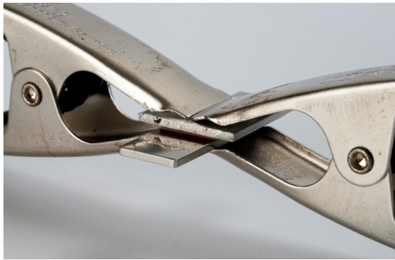
Figure 2.16: The clamping pressure is realized with two clamps via a metal plate (a). After curing of the adhesive, solder terminals are glued for establishing electrical contact to the strain gauge using enameled copper wires. A silicone rubber is used to seal the installation and protect against environmental influences (b).
