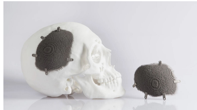
Figure 1.2: Examples for integrating of functionality through design: (a) Mold with integrated conformal cooling channel that is manufactured using metal based AM-processes [image source: www.desktopmetal.com ], (b) Tailored cranial implant made out of titanium [image source: www.eos.info/en ].
