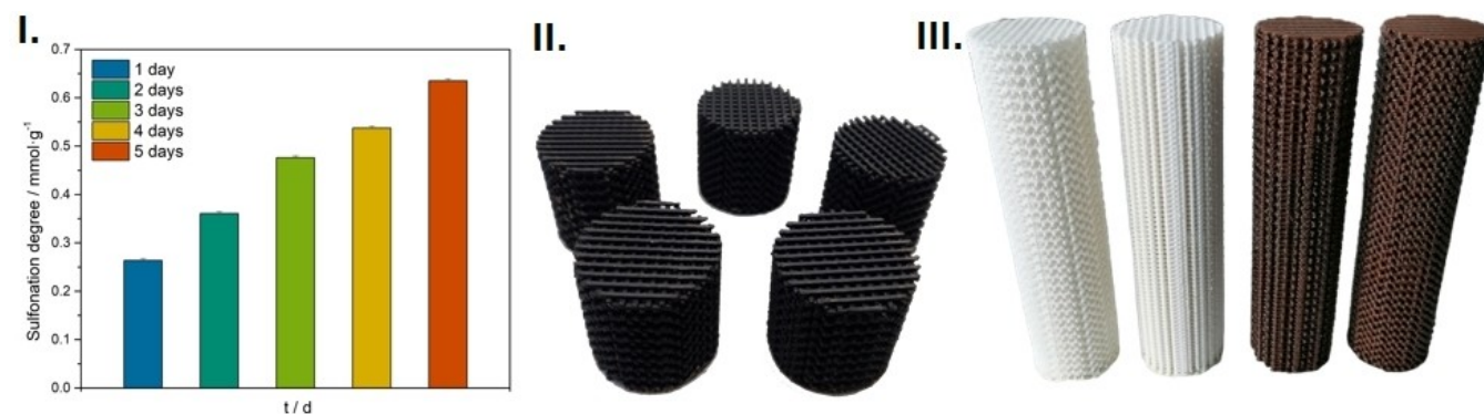
Figure 4. I. Time dependency of the sulfonation of HIPS monoliths of 1–5 days; II. A batch of HIPS monoliths after three days of sulfonation; III. ABAB and ABCD monoliths before (left) and after (right) sulfonation in sulfuric acid at 22 °C for 1 d.
