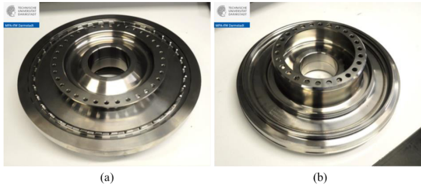
Figure 4.1 High pressure turbine disk made of Udimet 720Li used for specimen extraction [4.1]: (a) Top view; (b) Bottom view.
