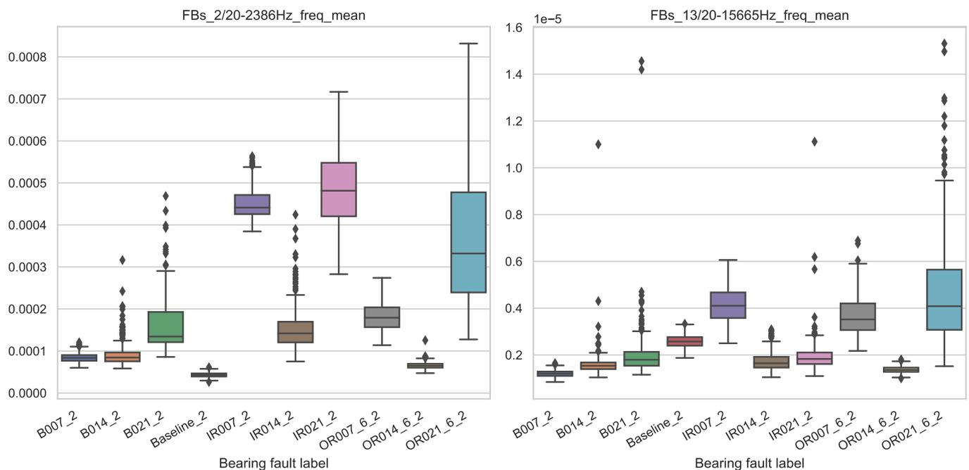
**Figure 7.** Box plot of feature value distributions over the different classes for the most important feature (**left**) and least important feature (**right**) from feature set FB\_20\_FD-mean.
