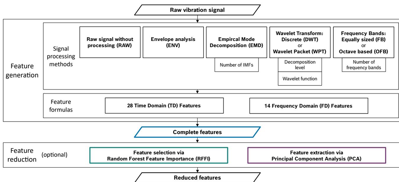
Figure 2. Modular design of feature engineering.
