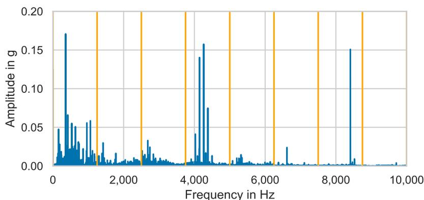
**Figure 1.** Equally sized frequency band separation (orange) of amplitude spectrum (blue).
