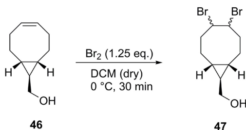
Scheme 53 | Synthesis of ((1R,8S,9R)-4,5-dibromobicyclo[6.1.0]nonan-9-yl)methanol 47 .
