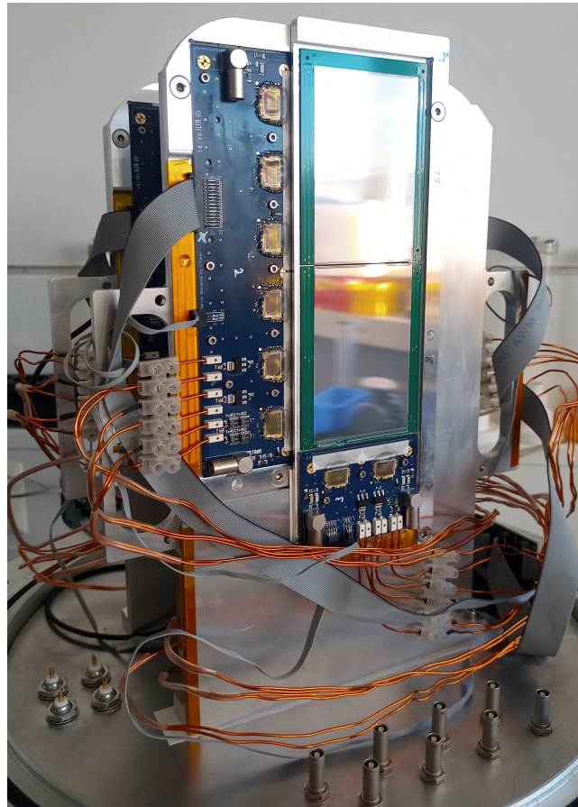
Figure 4.5: Picture of the PFAD silicon tracker assembled at TU Darmstadt.
