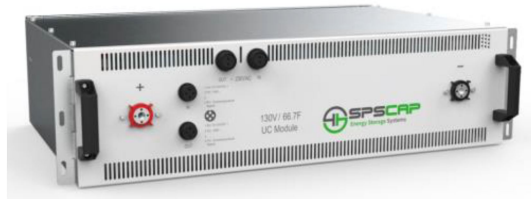
Figure 5.1: Supercapacitor module used for the prototype: the module is composed by 48 x 2.7 V cells in series for a total voltage of 130 V. Being a custom module built for this project, it has been decided to keep it as simple (and passive) as possible avoiding any active electronics in it (e.g. voltage balancing).
