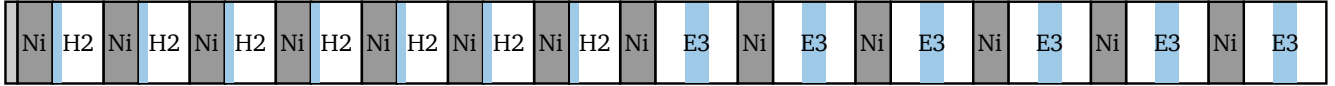
Fig. 2.2: RCF stack configuration for the TNSA source characterization during an experimental campaign with the LIGHT beamline in January 2021.
