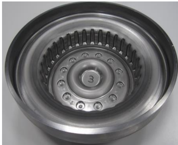
Figure 4 Clutch hub after gear forming (Source: ZF Friedrichshafen AG)
