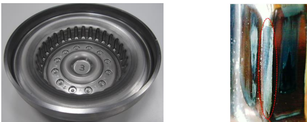
Figure 75 Left: clutch housing; right: wear mark of the tooth (Source: ZF Friedrichshafen AG)
