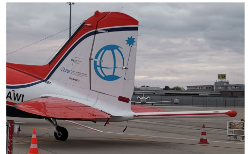
Figure 6.33: Magnetometer installed in the tail rod of Polar 5
