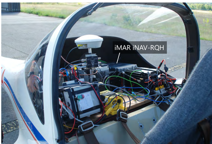
Figure 6.13: Installed gravimeters at ODW2017
