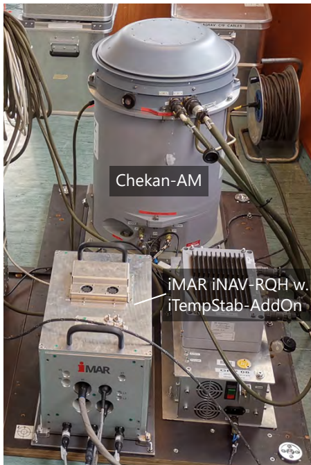
Figure 2.4: The Chekan-AM gravimeter owned by the GFZ installed next to TU Darmstadt's iMAR iNAV-RQH-1003 with iTempStab at the Müriz 2019 campaign
