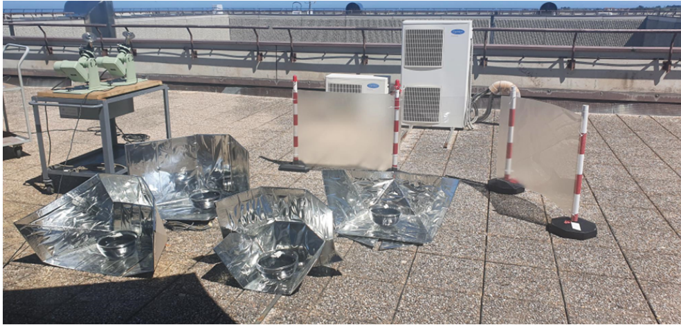
Figure 5.20: A picture of the four panels solar cookers placed side by side during a test with water with the wind shielding systems adopted.
