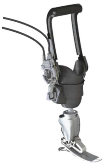
(a) Artificial gastrocnemius emulated with powered knee orthosis [44]
