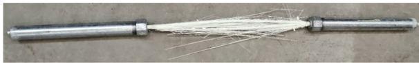
FIGURE 5 Typical failure mode of a GFRP reinforcement bar after reaching the tensile strength.
