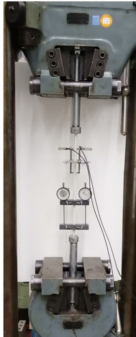
FIGURE 3 Short-term tensile test on a GFRP reinforcement bar in a universal testing rig.
