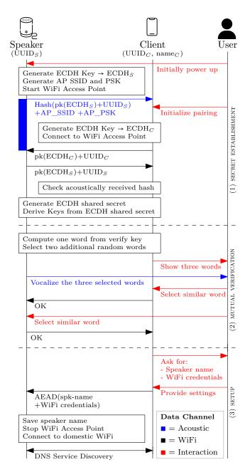
Figure 2: Pairing protocol for initial setup. pk(key) denotes the extraction of the public component from a keypair. MAC(message) denotes a keyed hash. AEAD(message) denotes an authenticated encryption. Hash(message) denotes a hash. All keyed algorithms derive keys from the ECDH shared secret. A bar denotes a recurring transmission until the next message occurs.
