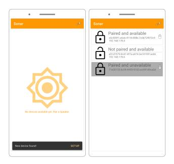
Figure 3: Primary App screen with no paired speakers (left), and with one paired and one unpaired speaker in the current WiFi network and a third unreachable paired speaker (right).
