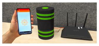
Figure 1: The user can securely setup a smart speaker. The pairing process involves an acoustic out-of-band channel to protect the integrity of the main channel.
