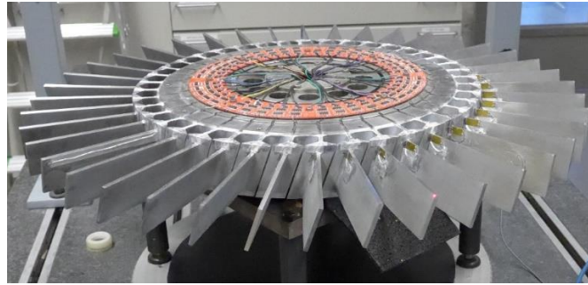
Figure 1: Test blisk of the Institute of Dynamics and Vibration Research (IDS), Leibniz University of Hannover.
