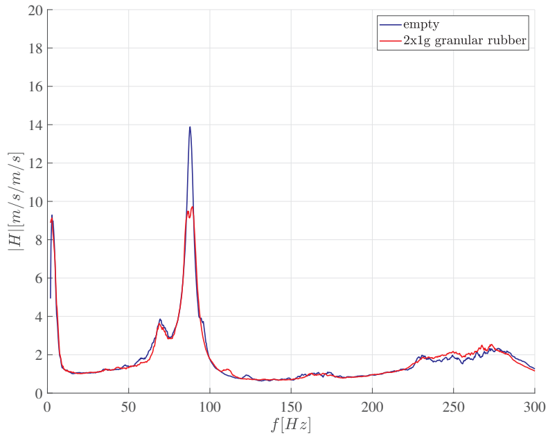
Figure 10: Frequency response at 180 rpm
