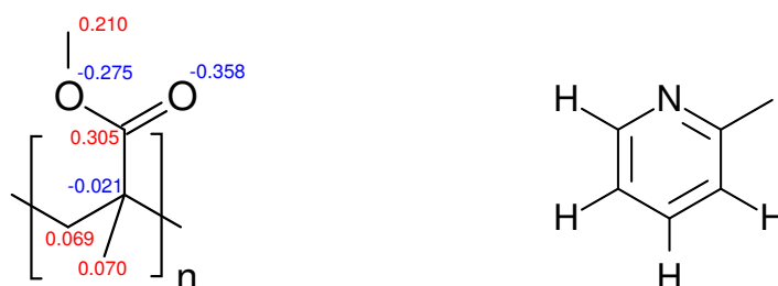
Figure 4.4.: Chemical formulas of the repeat unit of the polymer PMMA with modified partial charges (left) and the solvent 2-methylpyridine (right). Hydrogen atoms not explicitly shown are merged with their respective carbon atoms in the united atom force field. Created with BKchem by Beda Kosata.
