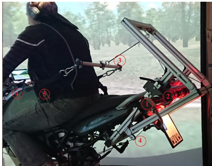
Figure 3.6: Rope Towing Mechanism of the DESMORI Simulator with ① DC Motor, ② Winch, ③ Back Connection to Rider, ④ Front Connection to Rider, ⑤ Manually Inflated Airbag Vest
