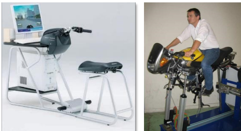
Figure 1.1: Honda Riding Trainer 2 as an example for simplified MRS for training purposes and hazard perception (left); IFSTTAR Motorcycle Riding Simulator 3 as an exemplary solution for MRS in the research and development domain (right)
