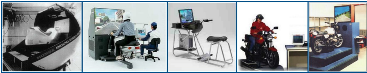
Figure 2.21: History of Motorcycle Simulators: l.t.r.: Honda First (4DoF) and Second (3DoF) Prototype, Honda Rider Trainer (Steering only), Kawasaki Motorcycle Simulator with HMD, Foerst Motorcycle Simulator with kinematic unstable mount.
