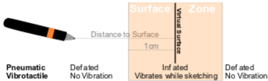
Figure P3.3: The unconstrained haptic assistance interaction technique combines vibrotactile and pneumatic feedback.
