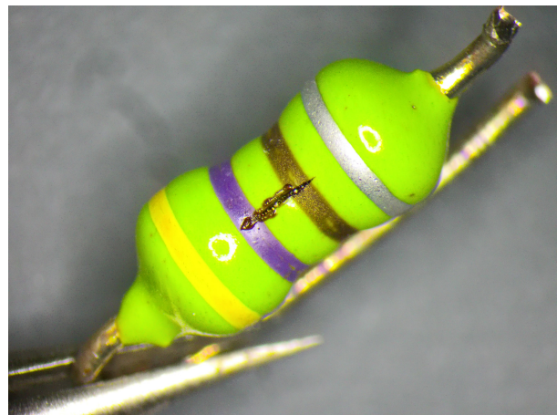
(b) Inductor with pin hole burn mark.
