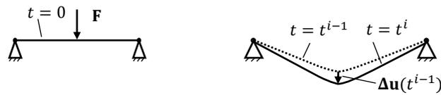
Figure 3.2: Different states of deformation in three-point bending illustrating the benefits of the DiESL approach (modified from Triller et al. 2021)
