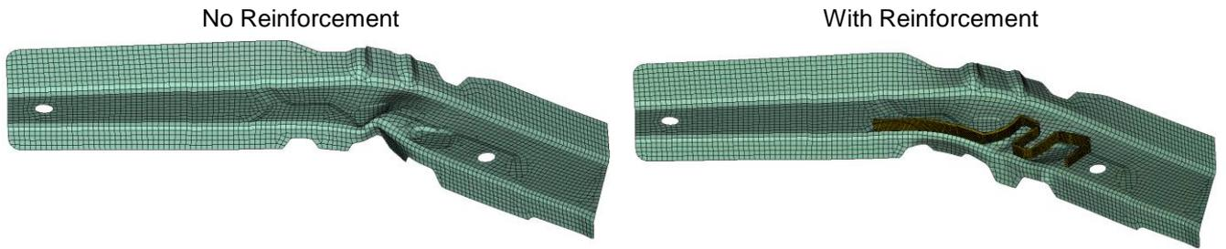
Figure 5.32: Reinforced Rail – maximum deformed rail with (right) and without reinforcement (left)
