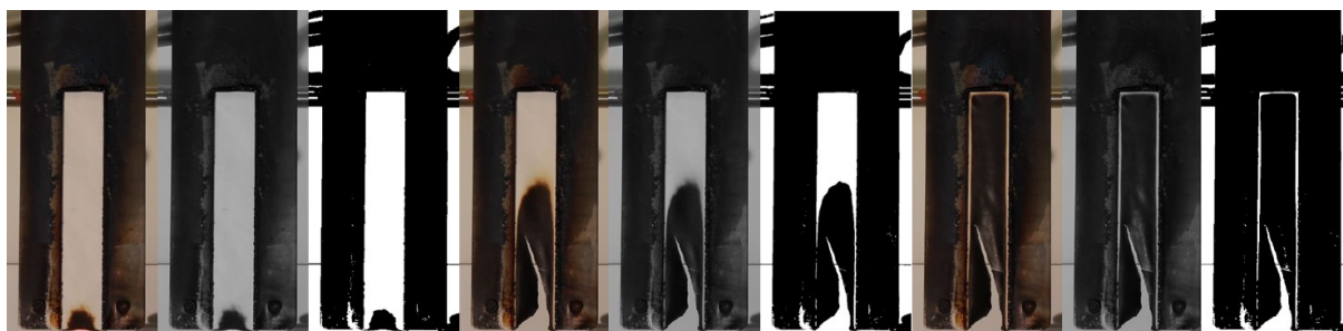
Figure 16: Conversion of the recorded picture stacks into black and white images.
