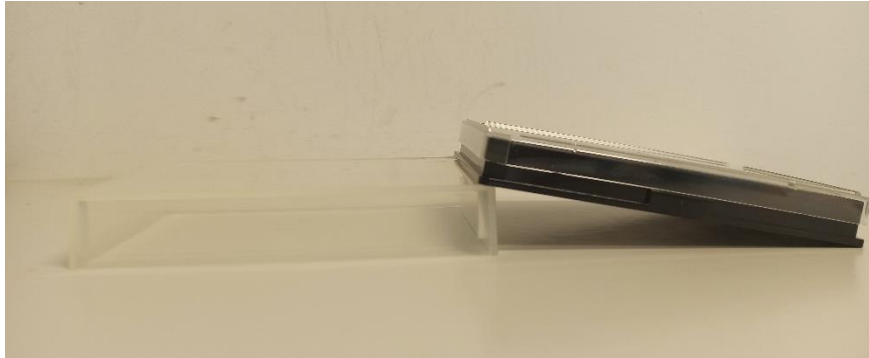
Figure 34: Plate position during incubation and wash steps for Immunofluorescent stainings of the OrganoPlate®. Every 2 min the positions was changed to the other side, to achieve a flow.
