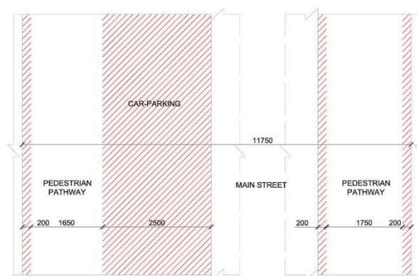
Figure 117: Street width and buffer spaces (in mm) for S2 gateway in residential area of Komponistenviertel in Darmstadt
