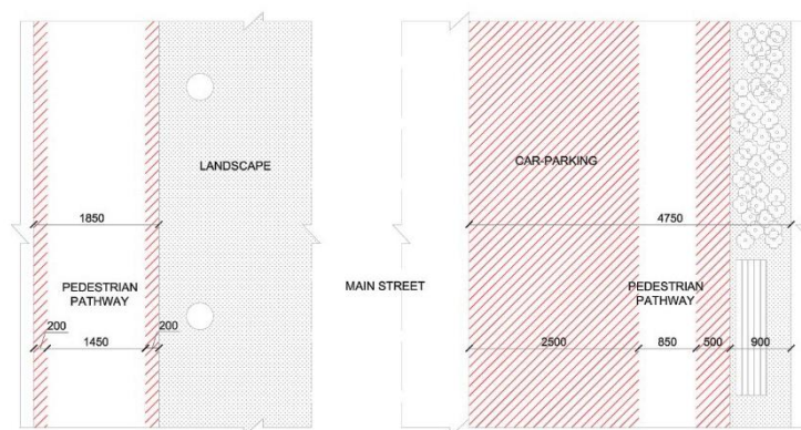
Figure 114: Street width and buffer spaces (in mm) for FS gateway in residential area of Komponistenviertel in Darmstadt
