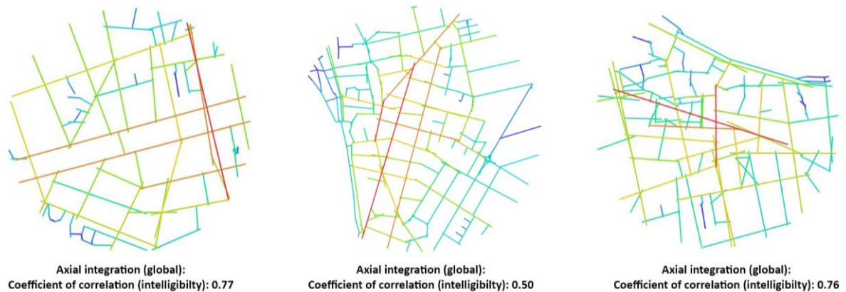
Figure 73: Global axial integration and relative intelligibility coefficient of axial lines surrounding Offenbach Hauptbahnhof (left), Bürgel (centre) and Marktplatz (right) within 1 sq. km.
