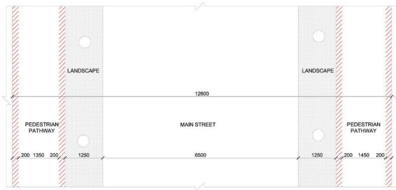
Figure 115: Street width and buffer spaces (in mm) for FN gateway in residential area of Komponistenviertel in Darmstadt
