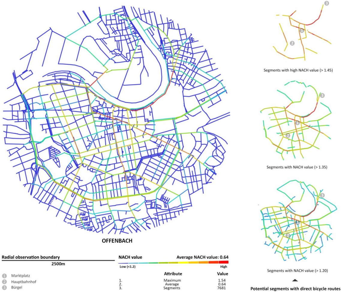
Figure 81: Segment maps showing normalisation of angular choice (NACH) through Offenbach within an observational radius of 2500m from the city centre i.e. Marktplatz
