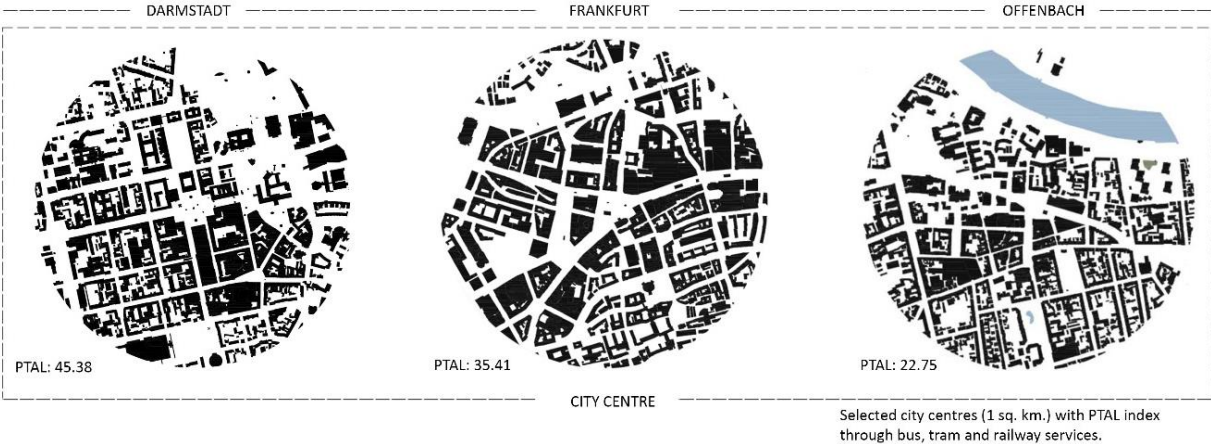
Figure 88: Figure ground maps of the city centres in Darmstadt, Frankfurt am Main and Offenbach am Main with corresponding PTAL values
