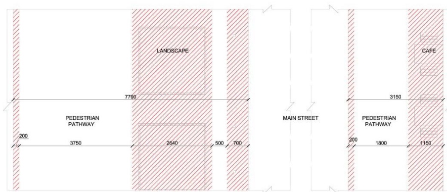
Figure 162: Street width and buffer spaces (in mm) for Gateway 2 in the area surrounding Frankfurt am Main Hauptbahnhof
