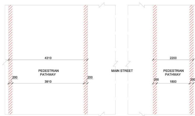
Figure 164: Street width and buffer spaces (in mm) for Gateway 4 in the area surrounding Frankfurt am Main Hauptbahnhof
