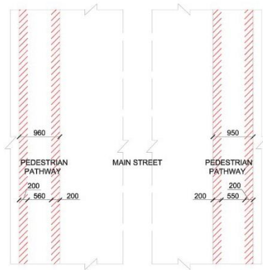
Figure 193: Street width and buffer spaces (in mm) for Gateway 6 in the residential area of Bürgel in Offenbach am Main
