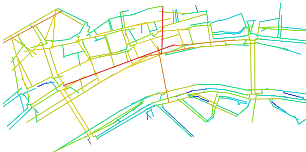
Figure 97: Local integration depicting the post-road closure condition of the Frankfurt Mainkai street
