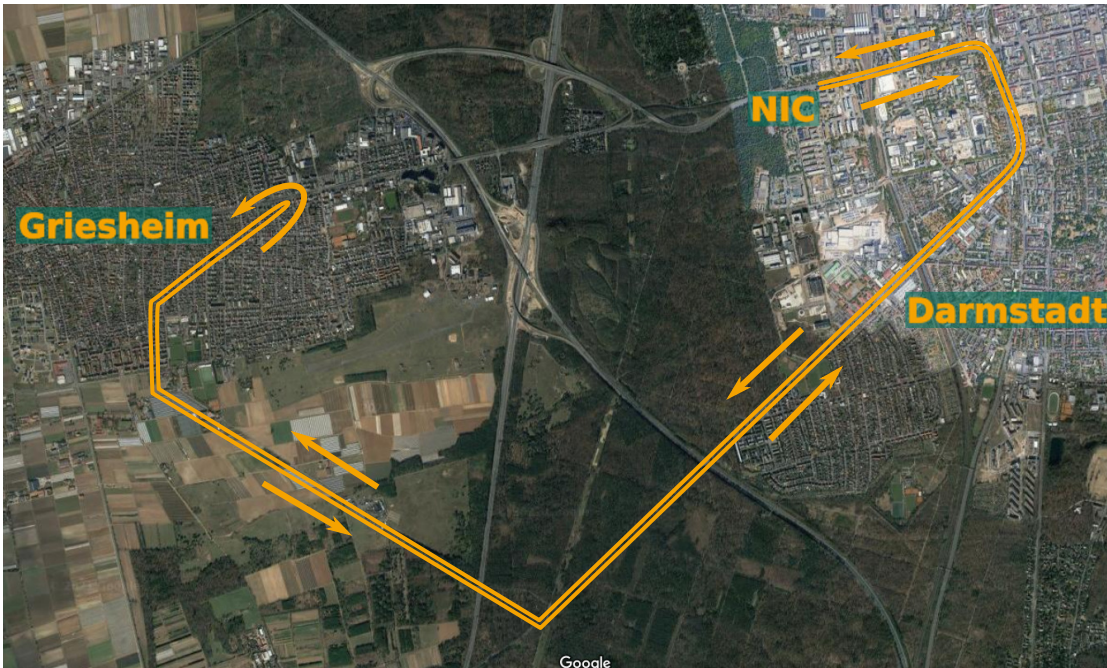
Figure 5.1.: Approximate route of the used optical communication fiber, deployed between Darmstadt and Griesheim. The qubits are generated in a lab at the Network Innovation Center (NIC) in Darmstadt, then sent to Griesheim, turned around there and detected again at NIC. Entangled qubits are detected directly at NIC, without leaving the lab. (Map source: Google Maps 2021 [158])
