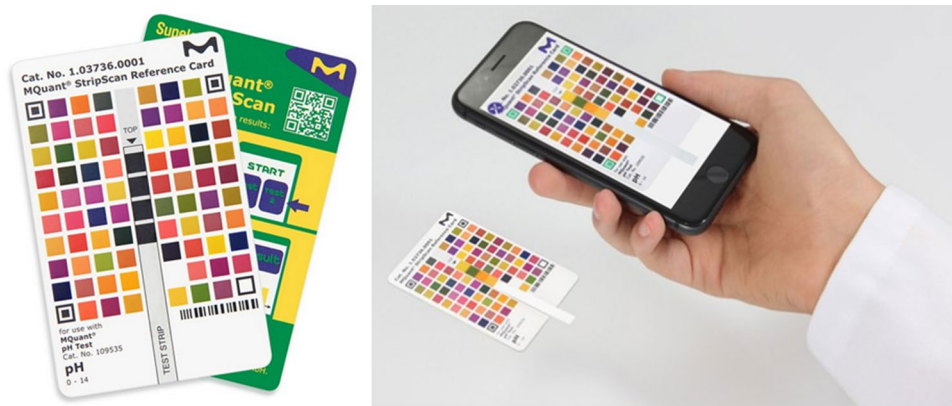
Fig. 24 The left image shows a reference card with space in the middle to place the dipstick. The right image shows the dipstick placed in the middle of the reference card and the use of the corresponding smartphone app. Reproduced with permission from [108]. Copyright Merck KGaA, Darmstadt
