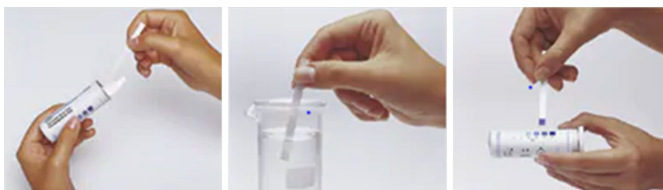
Fig. 13 From left to right. A dipstick is taken from the package. The test is performed. The strip is compared to a reference depicted on the package. Reproduced with permission from [65]. Copyright Merck KGaA Darmstadt
