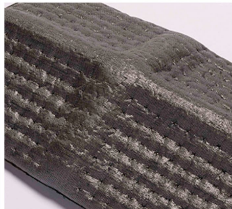
Fig. 8 Composite building component from expanded rPET particle foam in combination with lost form-work from rPET fiber—woven spacer fabric; left—planar element; right—self-foldable, formactive element. © Frankfurt UAS
