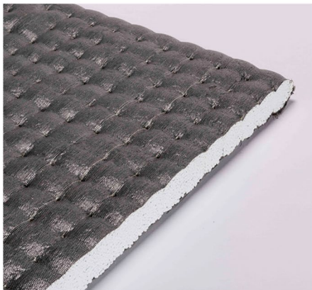
Fig. 8 Composite building component from expanded rPET particle foam in combination with lost form-work from rPET fiber—woven spacer fabric; left—planar element; right—self-foldable, formactive element. © Frankfurt UAS
