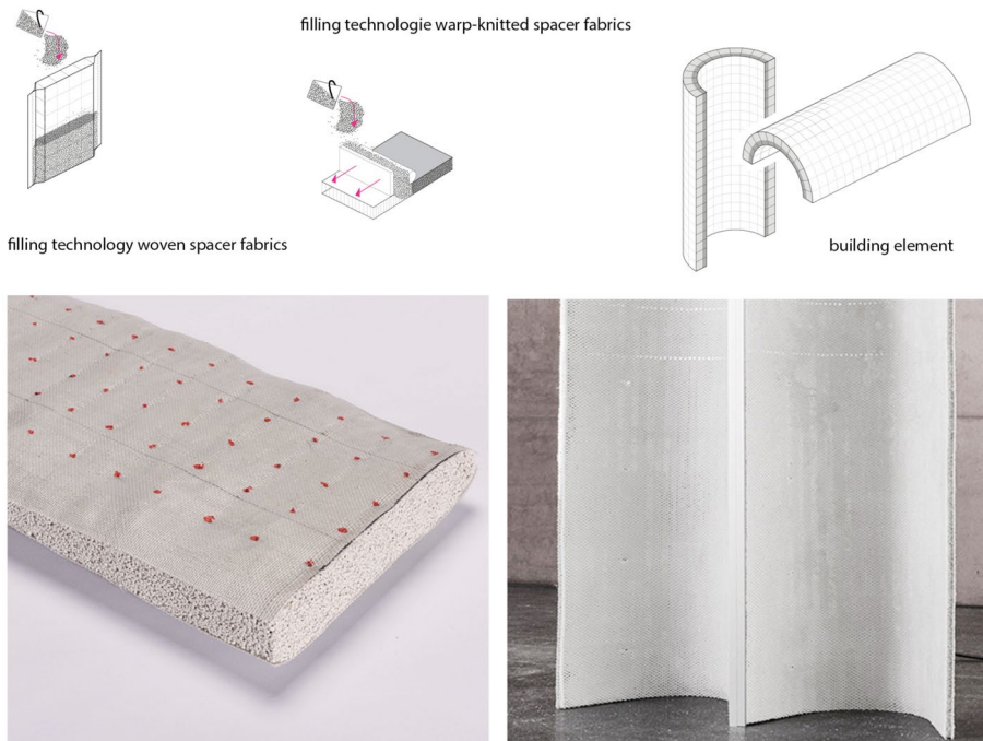
Fig. 7 Composite building component made of expanded glass in combination with lost formwork made of glass-fiber spacer fabric; below left - woven spacer fabric; below right - formactive warp-knitted spacer fabric. © Frankfurt UAS
