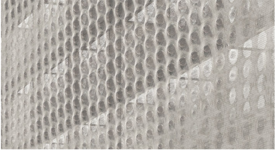
Fig. 12 ReFaTex, spacer textile, selectively stretched and in line with sunlight in real time with the help of internal pneumatic mechanisms. © Frankfurt UAS
