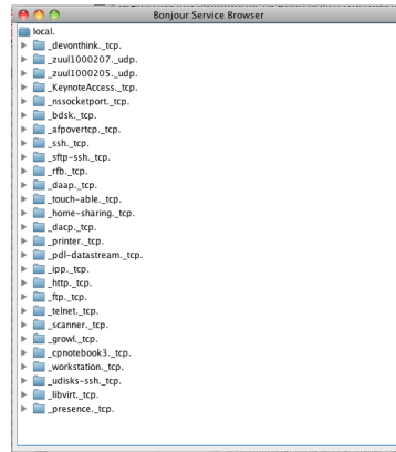
Figure 4.3: A Simple Network Service Discovery Browser combining 3 different service discovery mechanisms.
