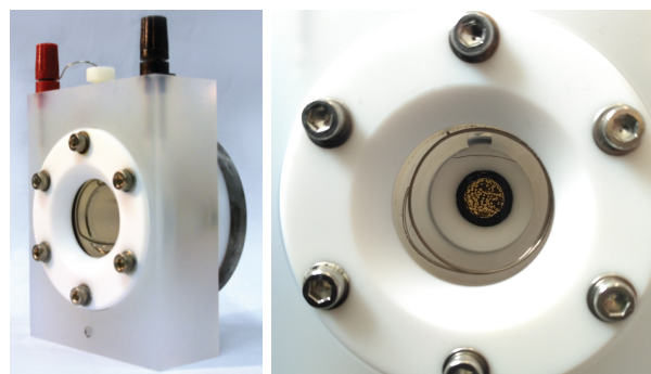
Figure 4.5: Left: Photography of the Photoelectrochemical Cell (PECC-2) from ZAHNER-Elektrik GmbH & Co. KG. used for EC measurements in this work. The cell is build for a three-electrode setup. A window allows observation of the sample during measurements. Right: Picture of a Au sample inside the Zahner cell during O 2 evolution, displaying air bubble adsorption on the surface of the sample.
