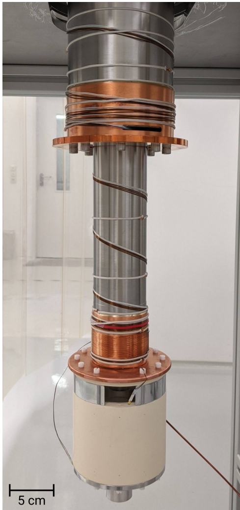
Figure 5.4: Complete sub-volume mounted to the tip of the cryocooler. On the left side of the volume the temperature sensor cable can be seen and on the right side the h.v. cable without ceramic beads.
