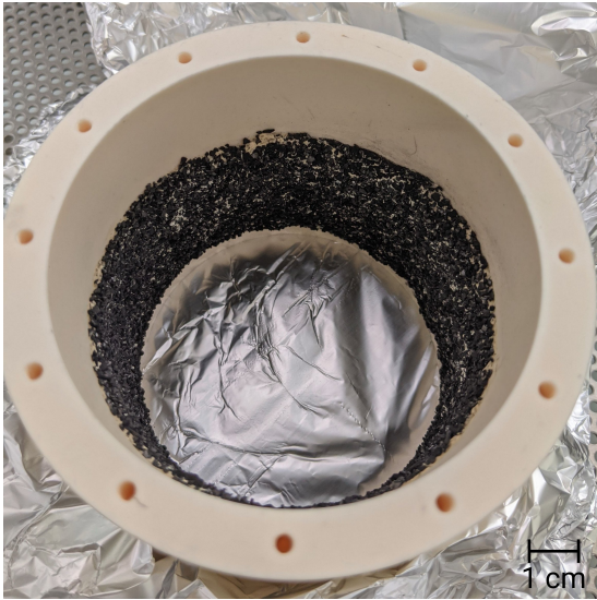
Figure 5.1: Sub-volume walls coated with activated charcoal.
