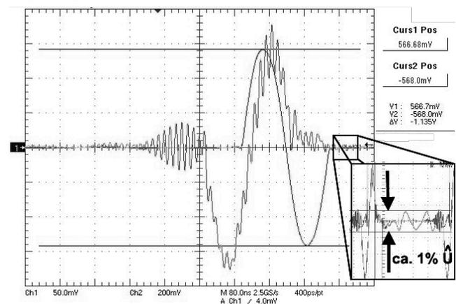
**Fig. 3:** pre-distorted input (jagged) and gap signal (smooth)
