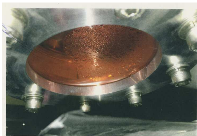
Figure 2.6.: Condensation water found during the experiment on the target entrance and exit windows. Courtesy Y. Sun.
