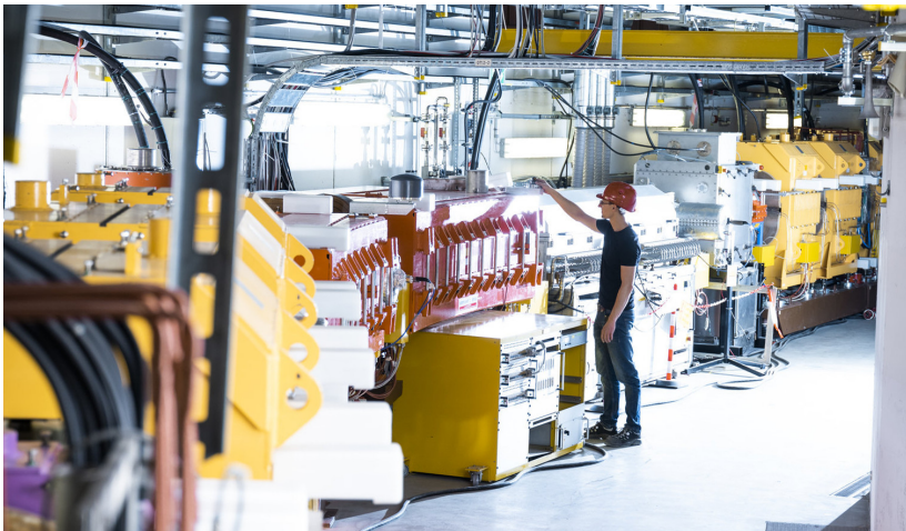
Figure 1.2: Magnets of the SIS18 synchrotron, dipole (red color, middle) and quadrupole (yellow color) magnets. The picture is adapted from [16].
