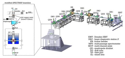
**Figure 1.** Schematic drawing of the HITRAP low-energy beamline (**right**) and a more detailed figure of the modified SPECTRAP beamline (**left**).
