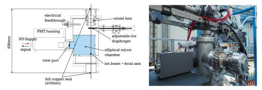
**Figure 2.** Schematic drawing of the optical detection region (**left**) and photo of the assembled vacuum system (**right**).
