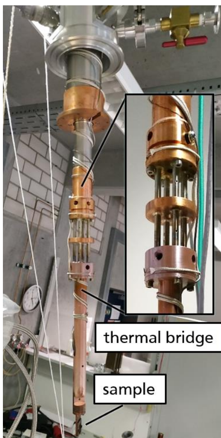
Figure 3.8.: Unmounted cryofurnace lifted with a Bowden cable. The inset shows the thermal bridge that prevents heating up of the first stage of the closed-cycle He cryostat while the sample is heated >300 K.
