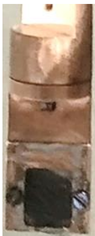
Figure 3.4.: Cold finger of the cryofurnace with flat sample clamped into a brass frame.
