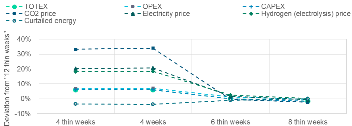
Figure 2-4 – Impact of the number of modeled representative weeks and the time interval compared to a twelve-week optimization in a carbon-neutral German energy system. ‘Thin weeks’ refer to a three-hour time step, and ‘weeks’ refer to an hourly time step.
