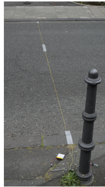
Figure 4.4.: Deployment of one electric field sensor on the street
