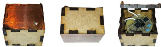
Figure 3.13.: ActiTag sensor housing top-front (left), front-bottom (middle) and top opened with ActiTag inside (right).
