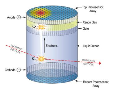
**Figure 4.** Principle of a dual-phase liquid xenon TPC. Energy from a particle interaction within the active liquid xenon volume produces prompt scintillation light (S1) and a delayed signal (S2) from electroluminescence (proportional scintillation) in the gaseous xenon layer. The localization of the S2 signal and the time difference between S1 and S2 allows for determination of the original vertex location.
